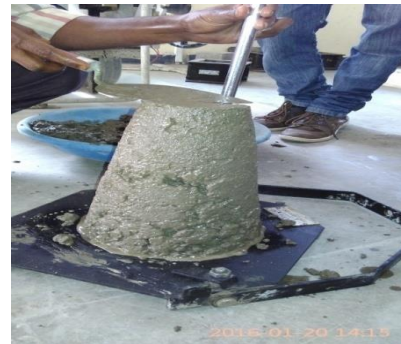
Figure 9. Slump Cone Test Of M40 Concrete
