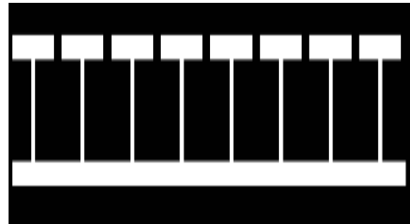
Figure 2: Mushroom like EBG Cross Section
