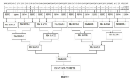
Fig 3.1: Block Diagram 8*8 bit High Performance Redundant Binary Multiplier
