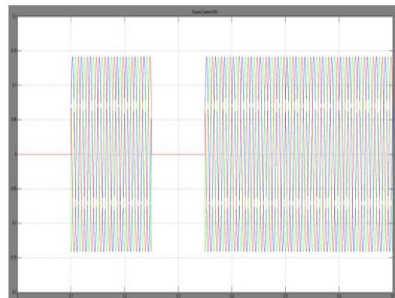
Figure 7 Source current drops and the THD of 2.57%
