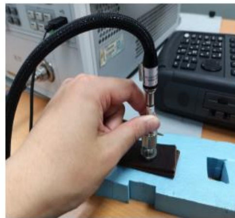
Figure 3-2 : The measurement setup for the electric properties of the leather.
